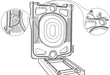
Fit the Ø 10.5 mm diameter thermocord into this U groove and into the groove which circles the furnace.
