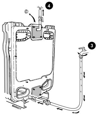
Ensure that all the air in the boiler is vented to avoid any bursting of the body.
