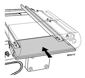
▶ Put in place the insulating material as shown above.
