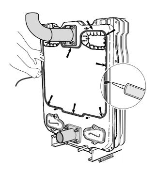
▶ Carefully insert the Ø 15 gasket in the groove of the rear section and hold it in place with a few drops of silicone.
