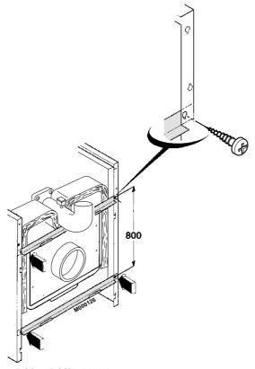
Put in place the 2 rear crosspieces (package RC2 or RC3)behind the bend of the rear side panels and fasten each crosspiece to the side panels using 2 screws ( $\emptyset$  3.94 x 12.7).
