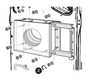
Close the furnace door on the 8 studs and fasten with 8 washers and nuts.
