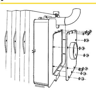
First adapt the steel connecting plate to the chimney connection flue, then fasten that plate or the plate with a connecting piece with 10 nuts H10 and Ø10 washers.
