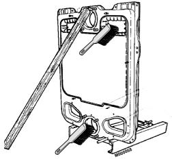
Clean all the openings in the section with a brush. Remove any deposit on the bottom of the section.
