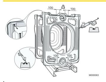
▶ Fill the bottom of the W groove opposite the U groove for the intermediary parts (located on the periphery of the section) with a continuous bead of DOW CORNING silicon, diameter approximately Ø 5 mm.
