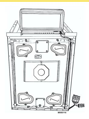
**b** Bring the **burner cable** behind the casing support and down to the burner between the side panel and insulating material.
