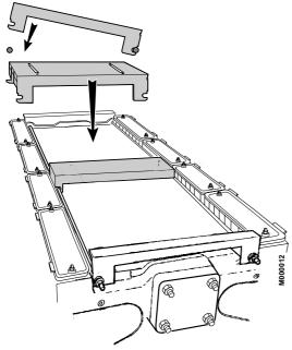
Assemble the intermediate piece on the assembly rods by fitting one slotted side onto one rod and using the flexibility of the other rod.
