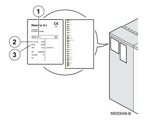
▶ Glue the rating plate and CE marking on the casing of the boiler in an easily visible location.
