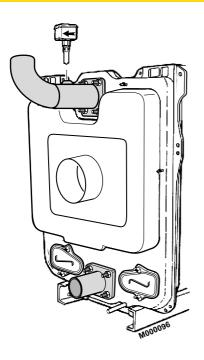
Fasten the flow switch on the sleeve tube. The direction of the arrow head on the collet must be the same as the flowing out of the water in the tube.
