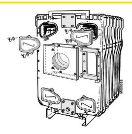
Fit the 2 doors of the upper flue ways (wing nuts).
