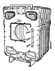
Fix the furnace door hinge on the right or left-hand side of the front section by means of 3 screws HM 12x25.
