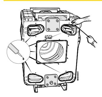
Insert the thermocord in the sealing groove on each side and hold it in place with a few drops of silicone filler.
