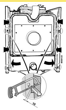
Put in place the insulation of the flue gas box and the lower rear insulating material (package RC2 or RC3).
