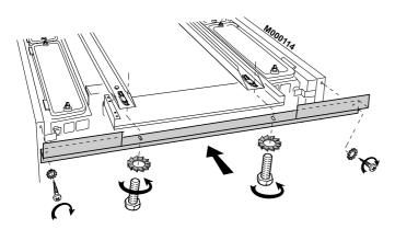
▶ Put the front crosspiece in place (package RC2 or RC3) and fasten with 2 screws (H8x16) and 2 tapping screws (Ø 3.94 x 12.7) + serrated washers.
