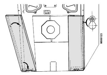
Fit the left and right-hand side front panels (package RC2 or RC3) onto the lower front crosspiece and fit them onto the studs of the side panels.
