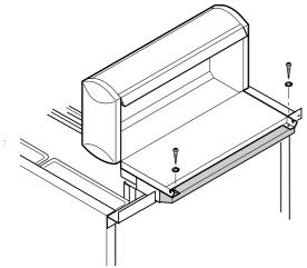
Fix the trim to the control panel using 2 tapping screws and serrated washers.
