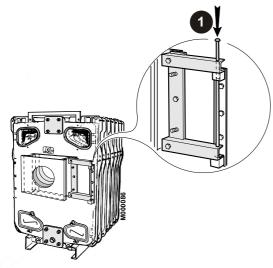
Fit the door onto the hinge by inserting the pin.
