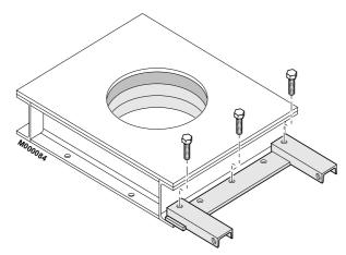
▶ Place the furnace door on the floor and fasten the articulation onto the door with 3 screws HM 12.
