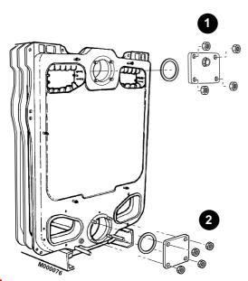
After assembling the boiler body, the installer must carry out a water tightness test at a pressure equal to 1.3 times the operating pressure (that is 9.75 bar mini) for 10 minutes at least.
