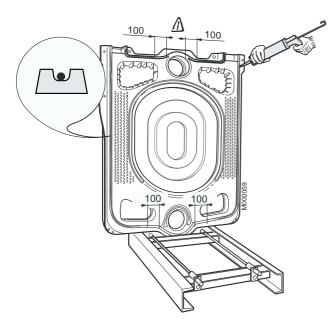
Fill the bottom of the U groove (located on the periphery of the section) with a continuous bead of DOW CORNING silicon, diameter approximately Ø 5 mm.
