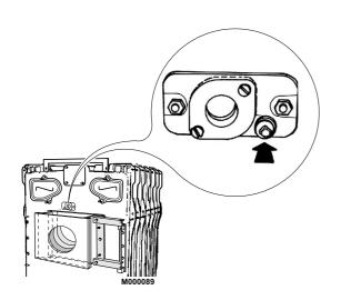
▶ The flame inspection window is fitted with a 1/4" tapped hole for ventilation (optional): if a ventilation system is used, connect the hole to the one provided for that purpose before the burner combustion head.
