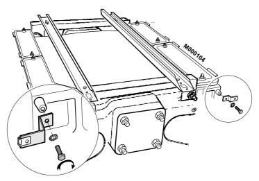
Fasten the positioning brackets (package RC2 or RC3) onto the right and left-hand upper bosses of the front section with: 2 screws H8 x 16 + 2 serrated washers (13 mm spanner).
