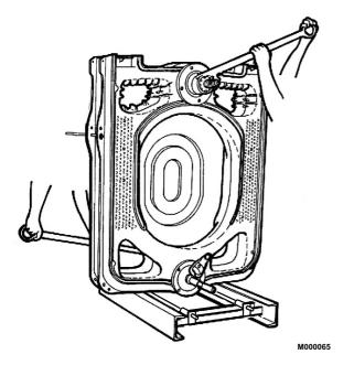
Put the assembly tool in position. Tighten gradually so as to bring together the upper and lower connections evenly and simultaneously.
